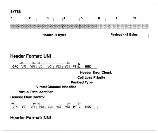
Figure 2. ATM UNI/NNI Format Data Cells
